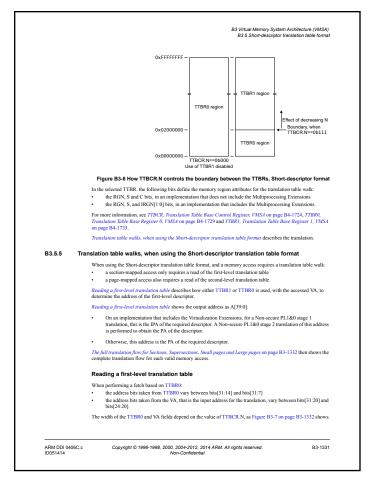
There are two page tables: one for the bottom portion of the address space (where the ukernel will live), and one for the top portion of the address space. What this documentation says is that the smallest bottom portion ends at 0x02000000 ... meaning a 32MB space.
