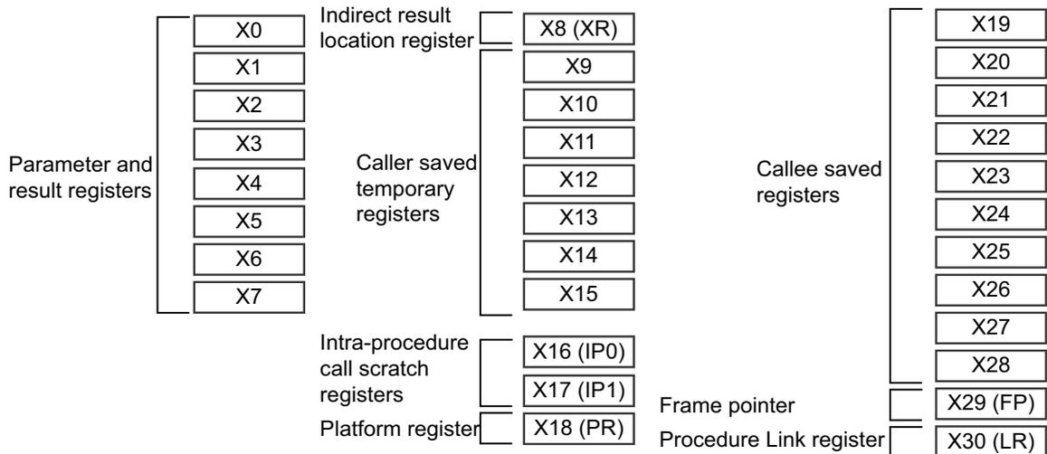
Figure 9-1 General-purpose register use in the ABI
