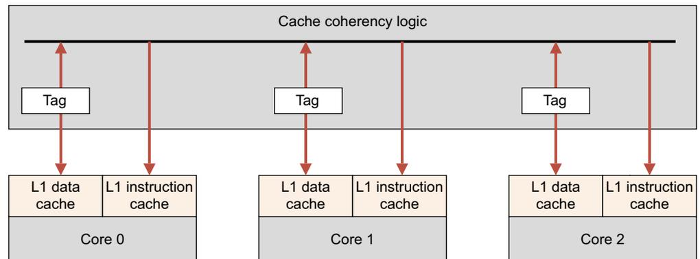
**Figure 14-4** Cache coherency logic
