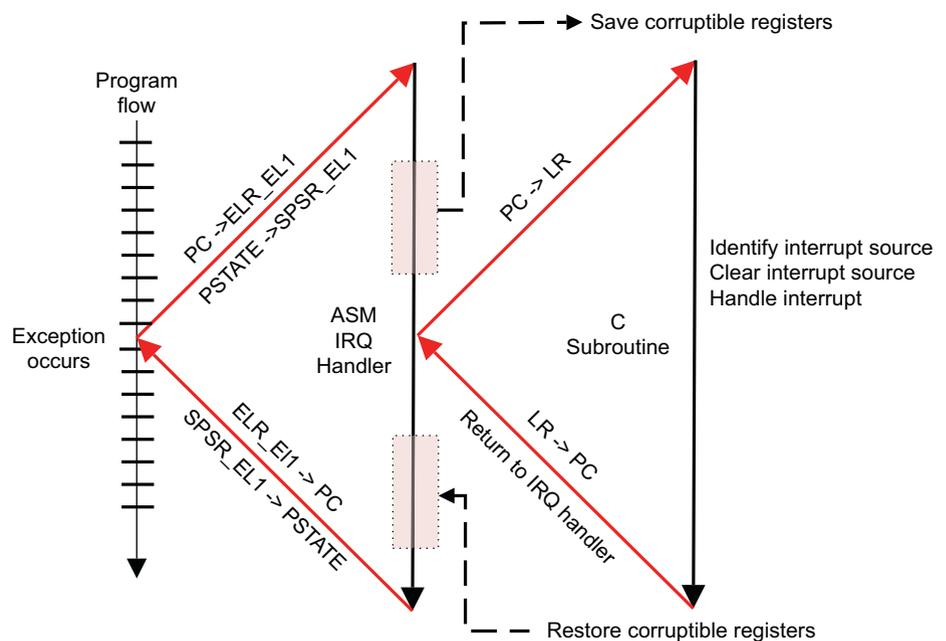
Figure 10-6 Interrupt handler in C code
