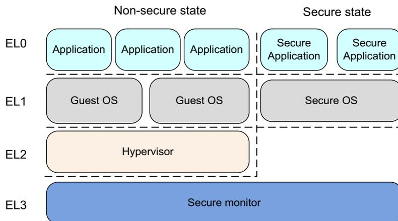
Figure 17-5 Security model when EL3 is using AArch64
