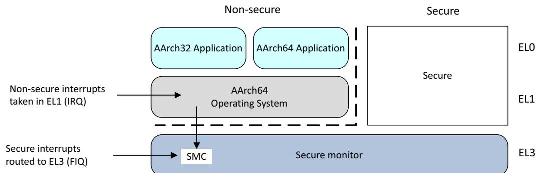
**Figure 17-1 Non-secure interrupts**
