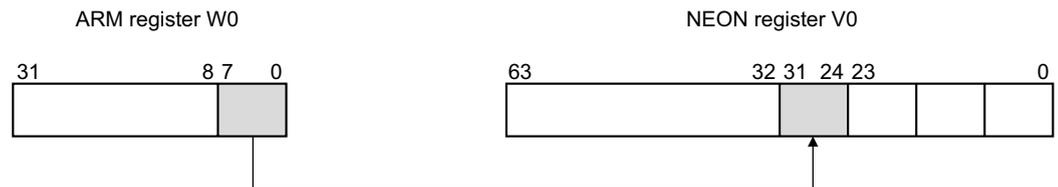
**Figure 7-5 Moving a scalar to a lane (MOV V0.B[3], W0)**
