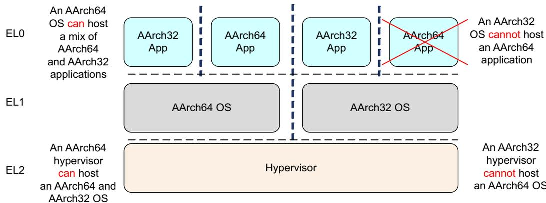
**Figure 3-7 Moving between AArch32 and AArch64**
