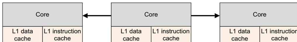
**Figure 14-3 Broadcasting cache operations to other cores**
