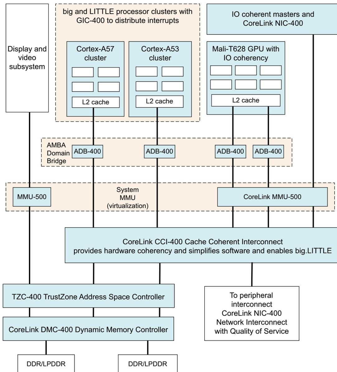
**Figure 14-8 Example mobile applications processor with CoreLink IP**
