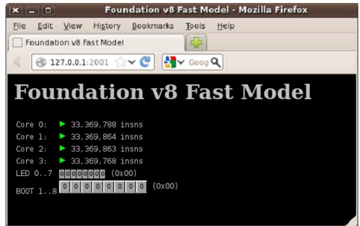
Figure 19-4 Multicore option with number of cores = 4
