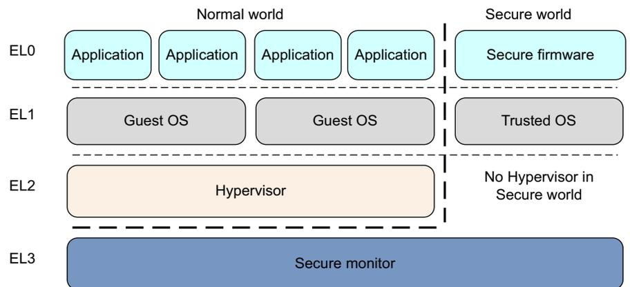
**Figure 3-2 ARMv8 Exception levels in the Normal and Secure worlds**
