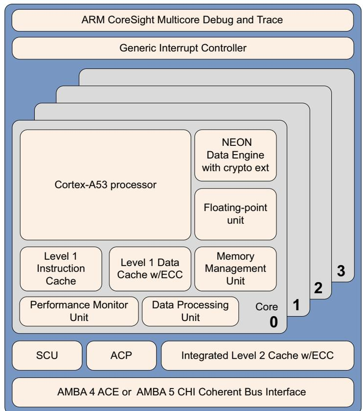
**Figure 2-2 Cortex-A53 processor**
