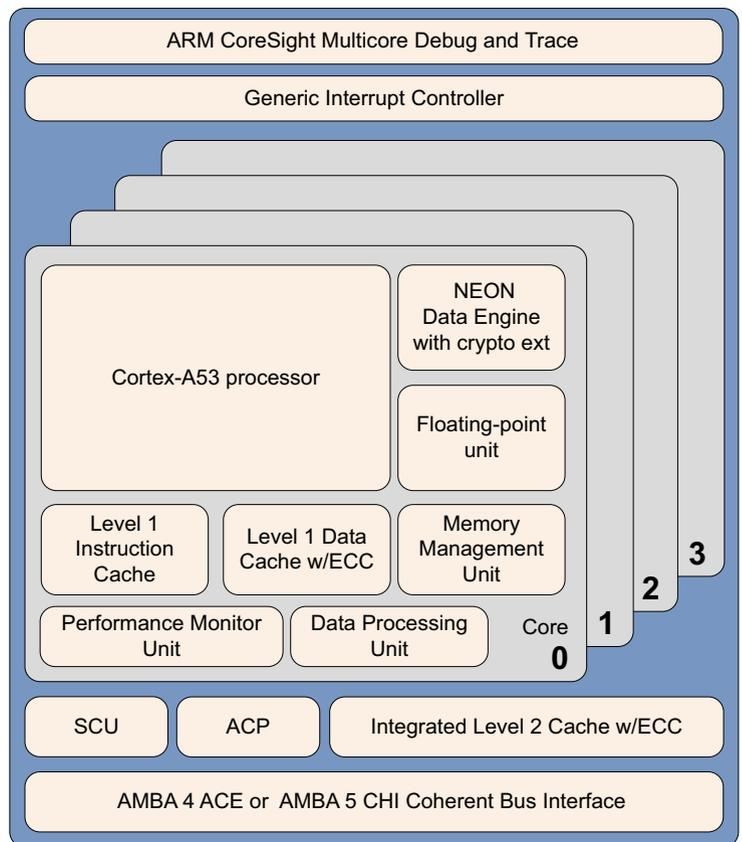
**Figure 2-2 Cortex-A53 processor**
