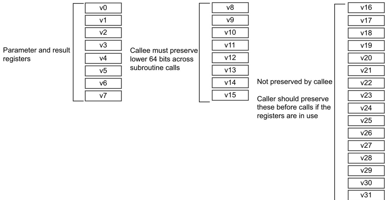
**Figure 9-3 SIMD and floating-point registers in the ABI**
