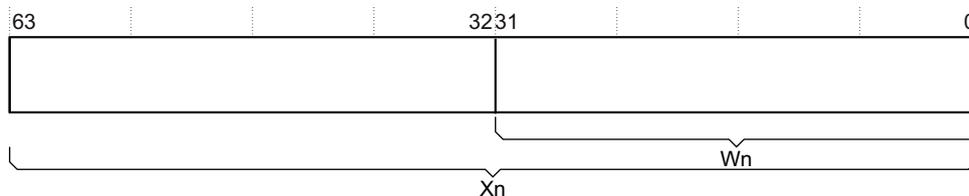
**Figure 4-2 64-bit register with W and X access.**
