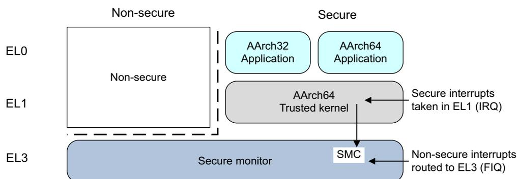
**Figure 17-2 Secure interrupts**
