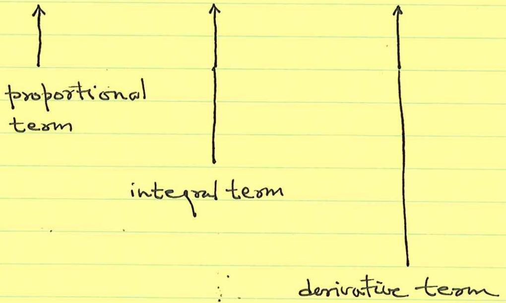
For suitable choices  $k_p, k_i, k_d$ , this linear controller, known as PID controller, reaps some of the benefits of feedback. The proportional term captures control based on present. The derivative term gives weight to the future (or predicted future) while the integral term draws on past error (or error history).
