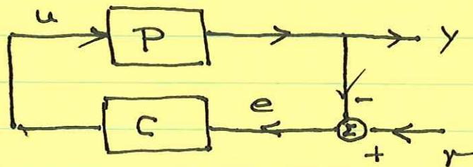
Here  $P$  denotes plant,  $C$  the controller, and the diagrams capture the equations
