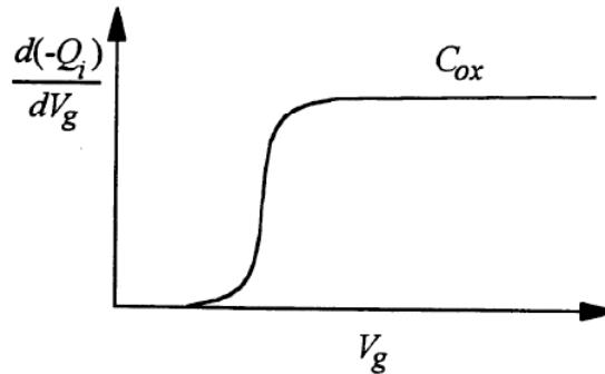
The sharp transition takes place at the threshold voltage.  $Q_i(V_g)$  is simply the integrated area under the above curve. Beyond threshold,  $Q_i$  increases linearly with  $V_g$  with a slope equal to  $C_{ox}$  (see Fig. 3.15 in the text).
