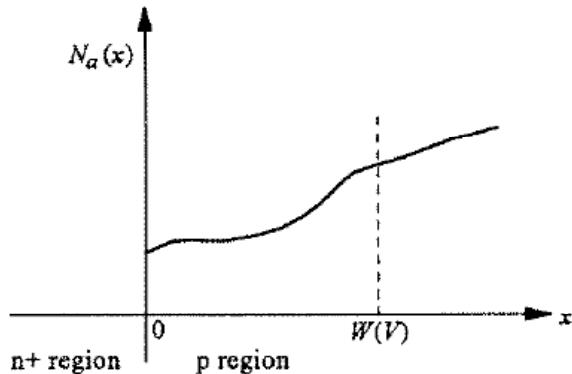
For the one-sided  $n^+$ -p diode, the incremental increase in the magnitude of the d layer charge  $dQ_d$  on the p-side as a result of an incremental increase in the applied voltage
