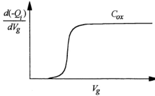
$Q_i(V_g)$  is simply the integrated area under the curve. Beyond threshold,  $Q_i$  increases linearly with  $V_g$  with a slope equal to  $C_{ox}$  (see Fig. 3.15 in the text).
