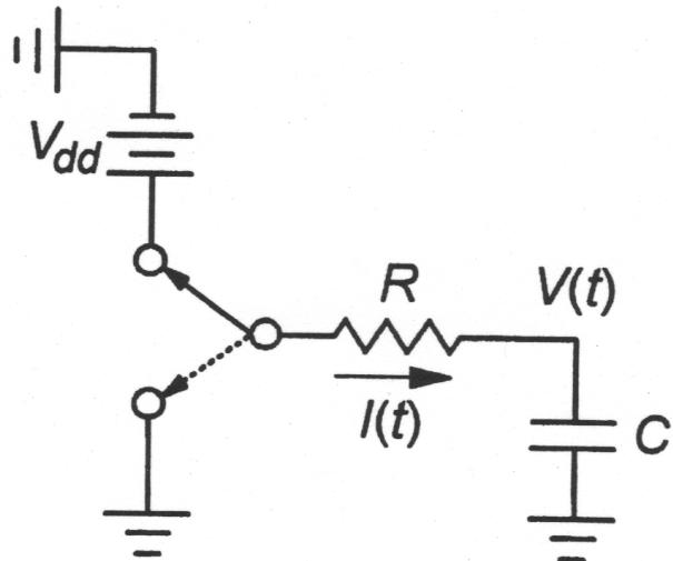
if the voltage source is switched to  $V_{dd}$  at  $t = 0$ , then
