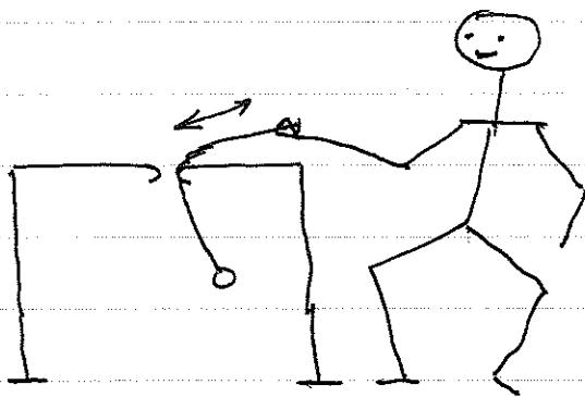
The pendulum is suspended on a string fed through a hole on a table top and controlled by an investigator.
