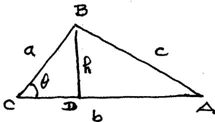
The area of a triangle with sides  $a, b, c$  is given by adding the areas of the two right triangles,  $BCD$  and  $BAD$ .
