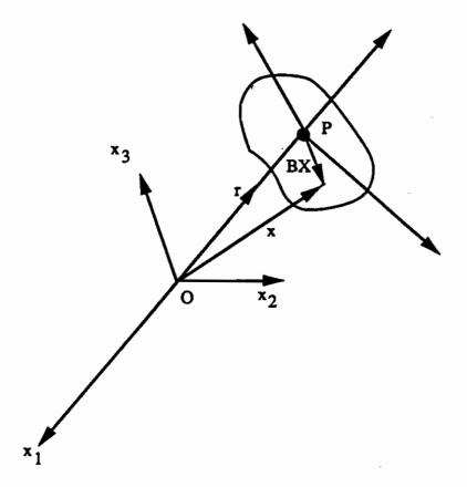
Figure 1.5.1 Rigid Body Kinematics
